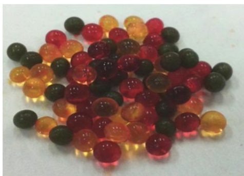
Fig. 1. Alginate-starch particles with encapsulated nicotine
