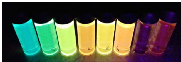
Fig. 1. Chromophore in different solvent (from left: hexane, toluene, dioxane, THF, chloroform, DCM, acetonitrile and acetone)
