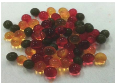
Fig. 1. Alginate-starch particles with encapsulated nicotine
